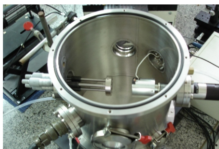
Figure 9. RPC like cell with a bulk aluminium anode and a glass cathode
