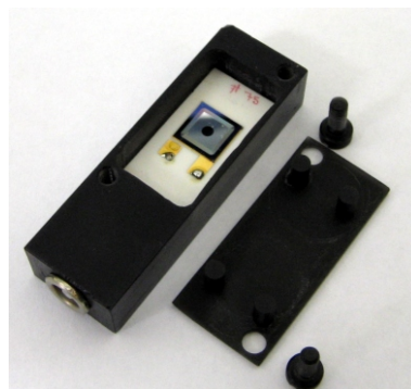
Figure 8. Magnetic Czochralski (MCZ) diode
