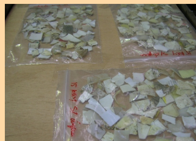
Figure 5. Irradiation of pesticides HDPE packing
