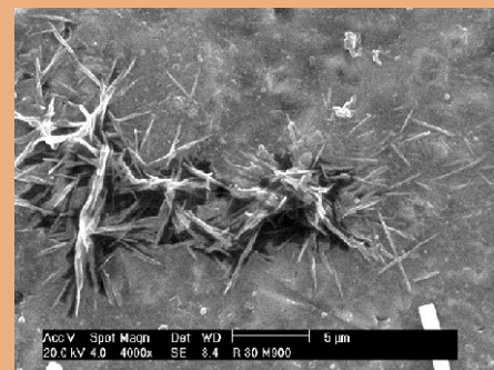
Figure 2. Fritted glass produced with 30 mass% WDR
