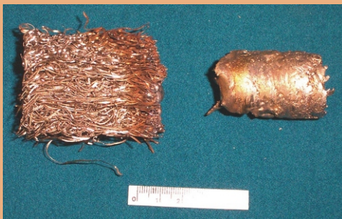
Figure 8. Macrograph showing a compact of stainless steel scrap and its consolidation in the VAR furnace
