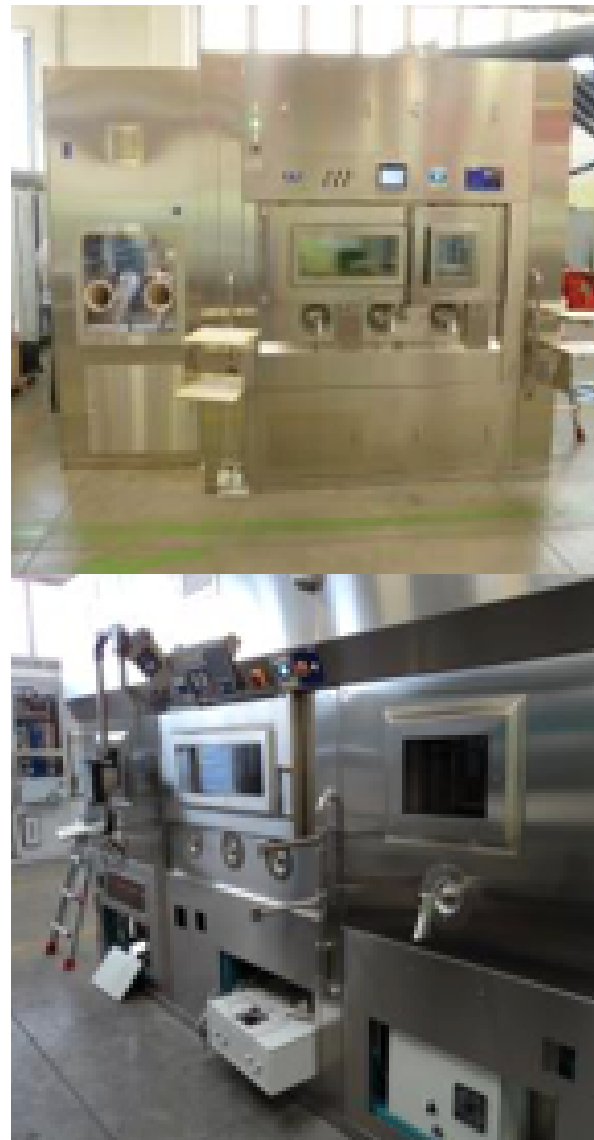
Figure 16a and 16b- New radiopharmaceutical production fractionating hot cells
