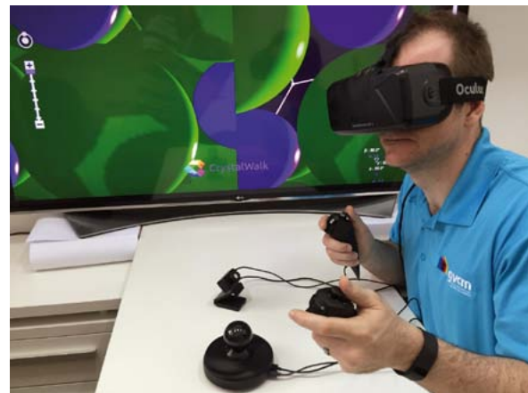
Figure 42: Advanced Interaction Support using Oculus Rift (head mounted display) and Razer Hydra (tracked joysticks).
