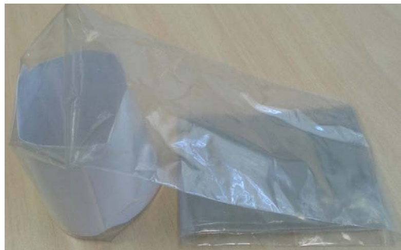
Figure 59. EVOH/GO (0.1 wt. % GO nanosheets Flexible Films.
