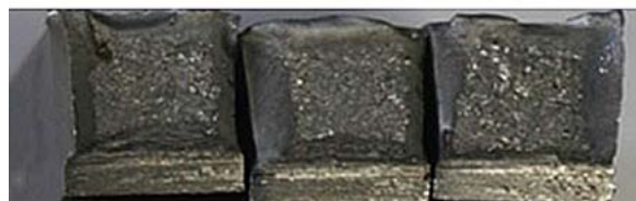
Figure 28: (a) Welded joint between tube and curve - Dimensions in millimeters (b) Influence of the tempering time in the various welding regions (c) Surface of the fracture region, the top sample without lateral expansion of the weld metal (WM-CS) and the bottom samples with lateral expansion of the weld metal (WM-8h) (d) Energy absorbed in the impact test x welded joint regions and (e) Lateral expansion in WM in the top and in the root.
