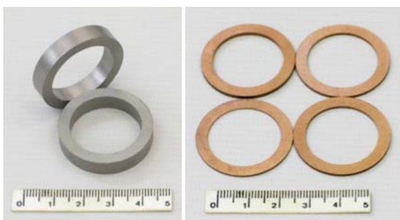
Figure 31: Copper rings (left) and inserts (right) before sintering process, respectively.
